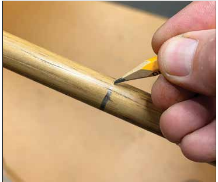
MARKING THE SHAFT is a great visual aid in helping the woodworker know how much or where you have filed, sanded, or scraped.
