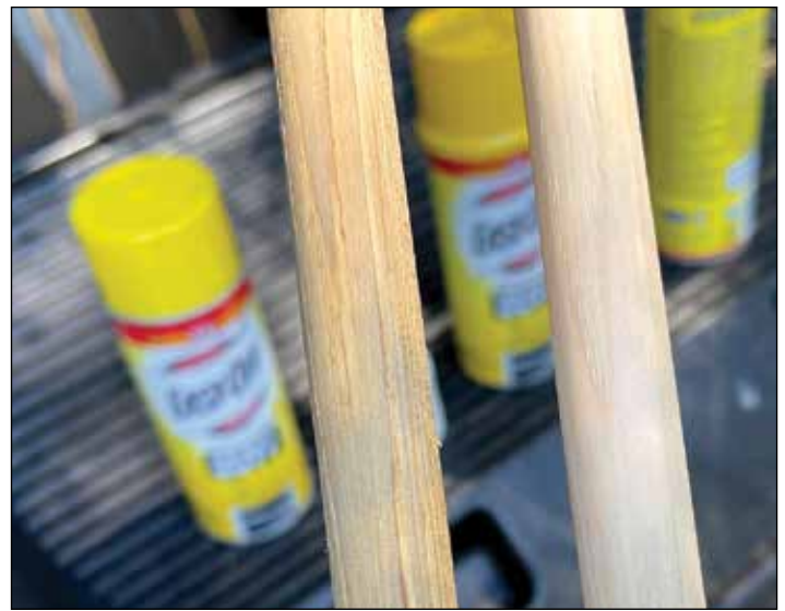
BEFORE AND AFTER SANDING. Tim Bell uses Easy-Off oven cleaner to oxidize the wood and raise the grain. The process helps him achieve the patina he desires.
