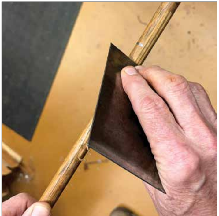
A LARGE STANLEY HAND PLANE BLADE does the trick for Tim Bell to scrape his hickory shafts.
