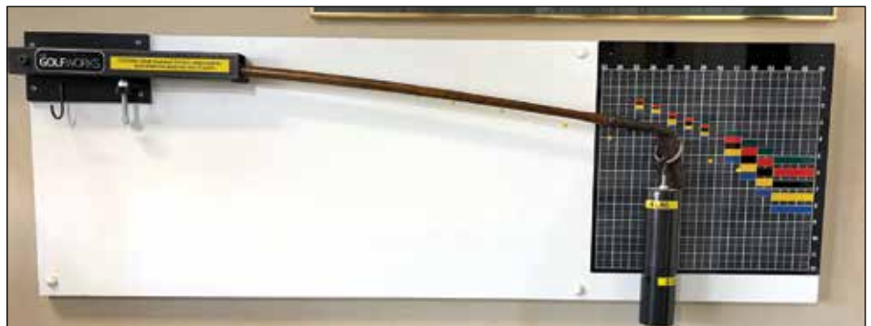
DEFLECTION BOARDS , such as this one from GolfWorks, allow club repair experts to measure the flex in hickory shafts. It is an impressive bit of workshop technology and is sure to wow hickory novitiates. Get two! (Photo courtesy Bill Geisler.)
