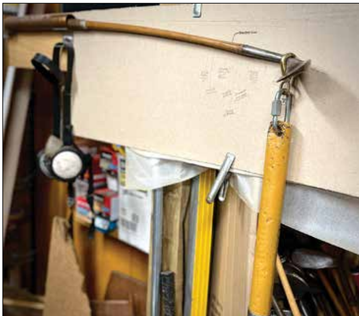
SHAFT FLEX BOARD with a calibrated weight tells the story of the flex of a shaft, stiff to regular, or points in between.
