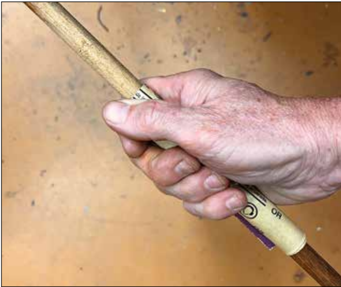
SANDPAPER WRAPPED AROUND THE SHAFT helps to remove rough wood fibers.
