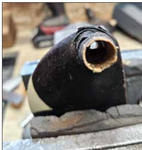
PHOTO 5. Drilled hosel after using reamer.
