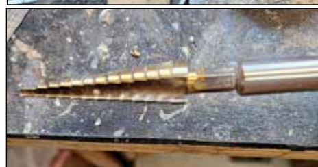
DRILL BITS FOR THE JOB. Top photo, a 1/2-inch tapered, step-down bit. Above, a 1/2-inch tapered reamer. You'll also want an extension bit for added length, like the one shown with the reamer.
