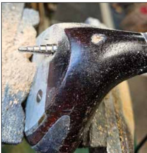
PHOTO 4. Bit extends past sole plate.
