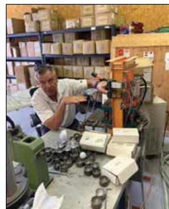
From the hand press, balls move to press that produces the necessary temperatures to create the surface patterns.
