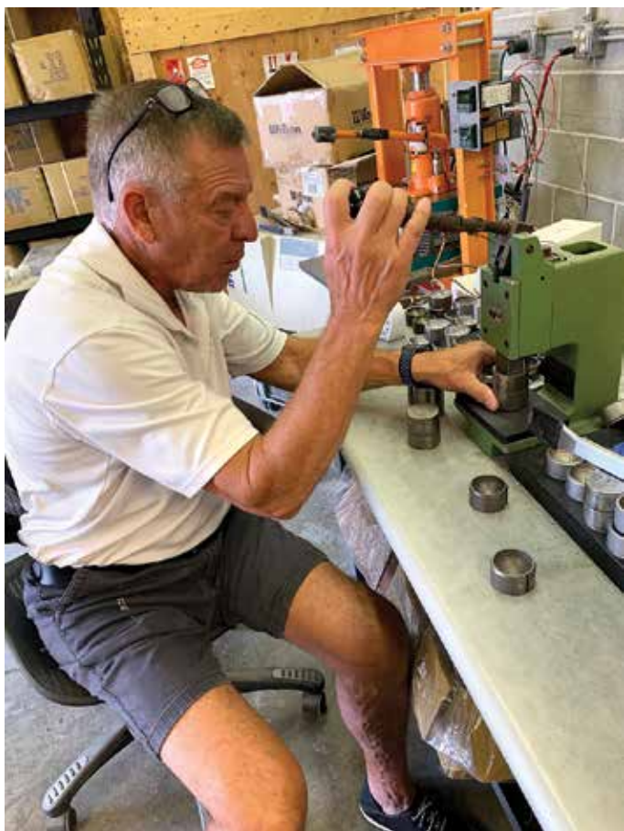
Using a hand press, balls are prepared for the heat and cold press using an original mold to achieve the desired surface pattern.
