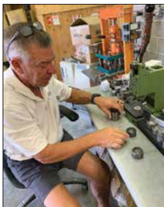
From the hand press, balls move to press that produces the necessary temperatures to create the surface patterns.
