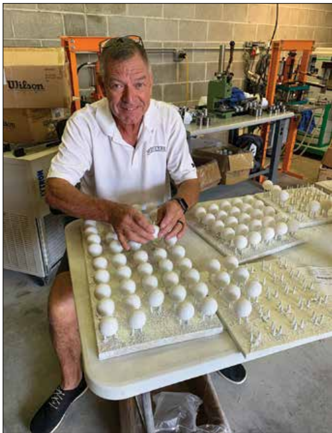
Dave Brown , the man who provides replica golf balls to the hickory golf community, in his shop with a rack of gutty balls during the painting process. “After trimming, they have to be rotated six times to ensure full coverage,” he says.
