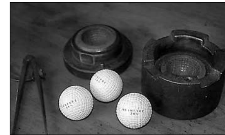
GUTTA PERCHA golf balls made from authentic 1880s line cut cast iron mold.
