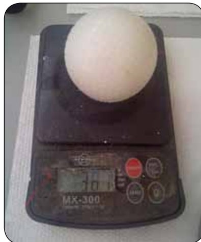
The McIntyre ball weighs 38.1 grams, 97% comparable weight to the organic sample. It is assumed that the organic gutta percha is slightly more dense, molecularly, to produce this result.
