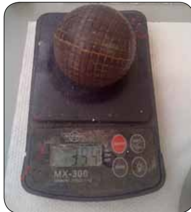
The organic ball with its ring removed weighs 39.4 grams.
